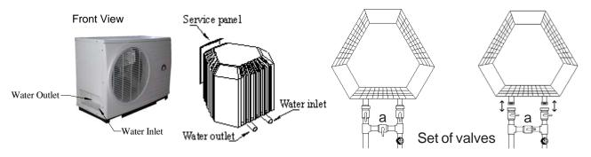
To adjust the water flow going through the pool heater, please adjust the by-pass valve (a) in the following way:
